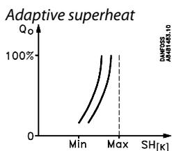
Regulation is based on evaporator load by establishing minimum stable superheat (MSS). The superheat reference is lowered to the exact point where instability begins. The superheat is limited by the settings for minimum and maximum superheat.
