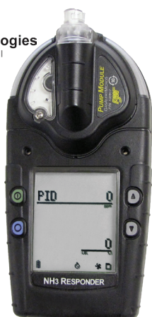
Specially configured GasAlert Micro 5 PID
